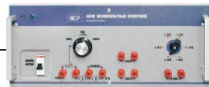
Low-voltage measurements unit
